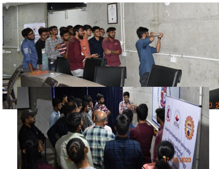
Pic- 7: Practical Session of NDT Schmidt Rebound hammer test
